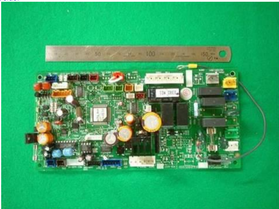
62.MMU-AP0074YH-E, MMU-AP0094YH-E, MMU-AP0124YH-E_ Control PCB _MCC-1403, component side.
