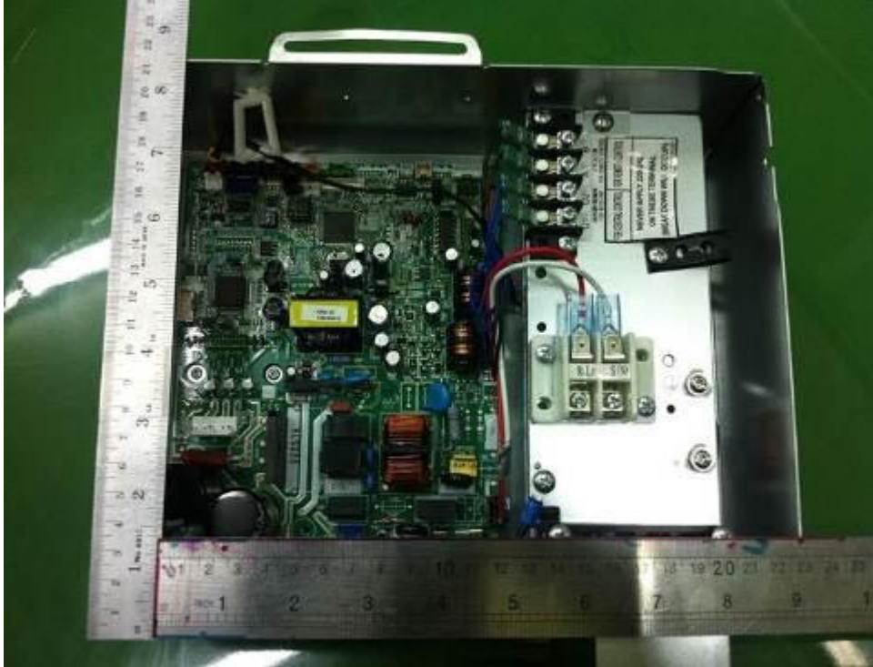
136.PCB of construction after removed cover for MMD-AP****HP-E.
