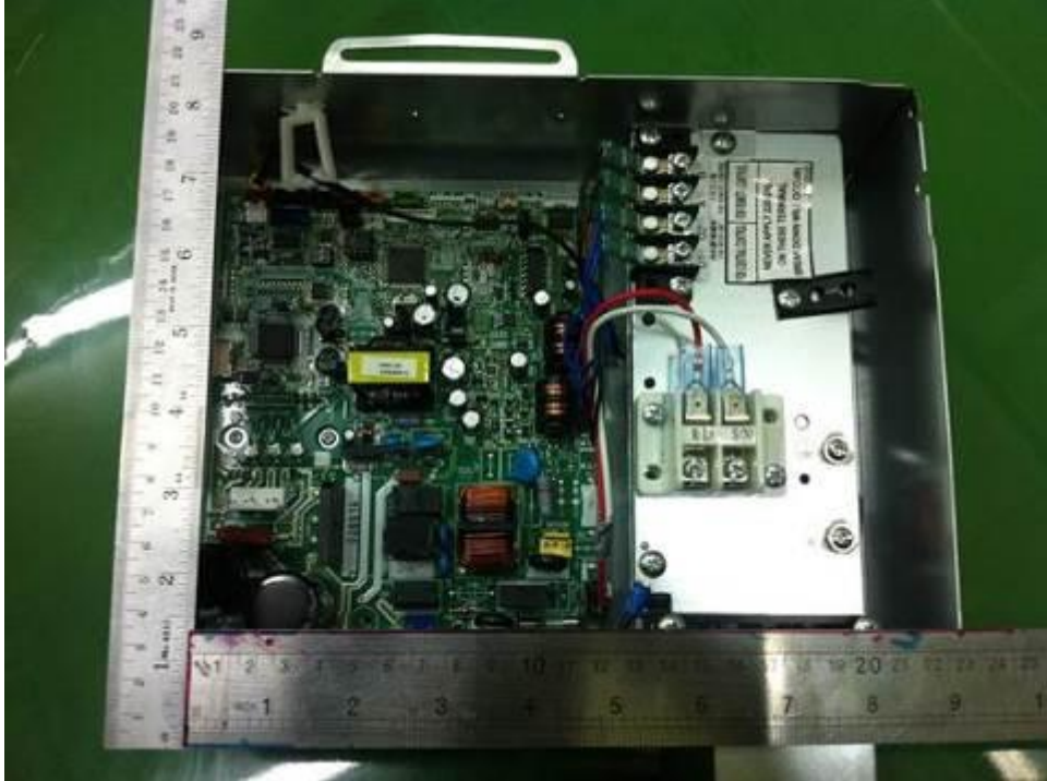
82.MMD-AP***BHP-E_PCB of terminals for connection of interconnection cord all indoor units.
