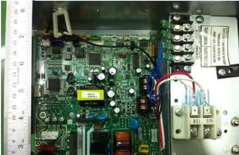
82.MMD-AP***BHP-E_PCB of terminals for connection of interconnection cord all indoor units.
