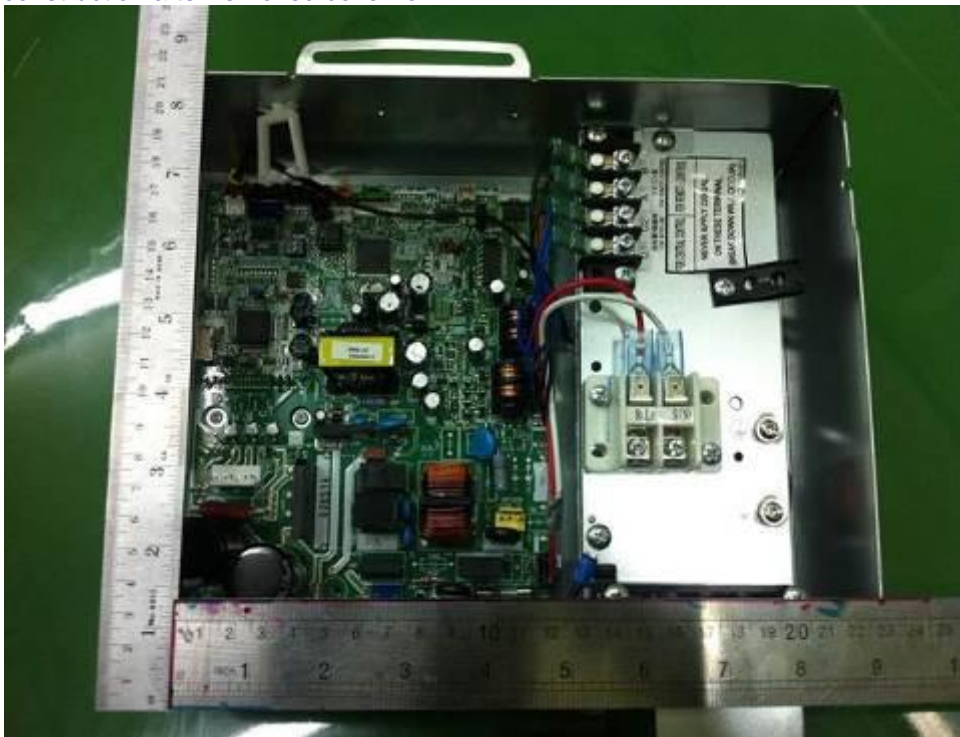
136.PCB of construction after removed cover for MMD-AP****HP-E.
